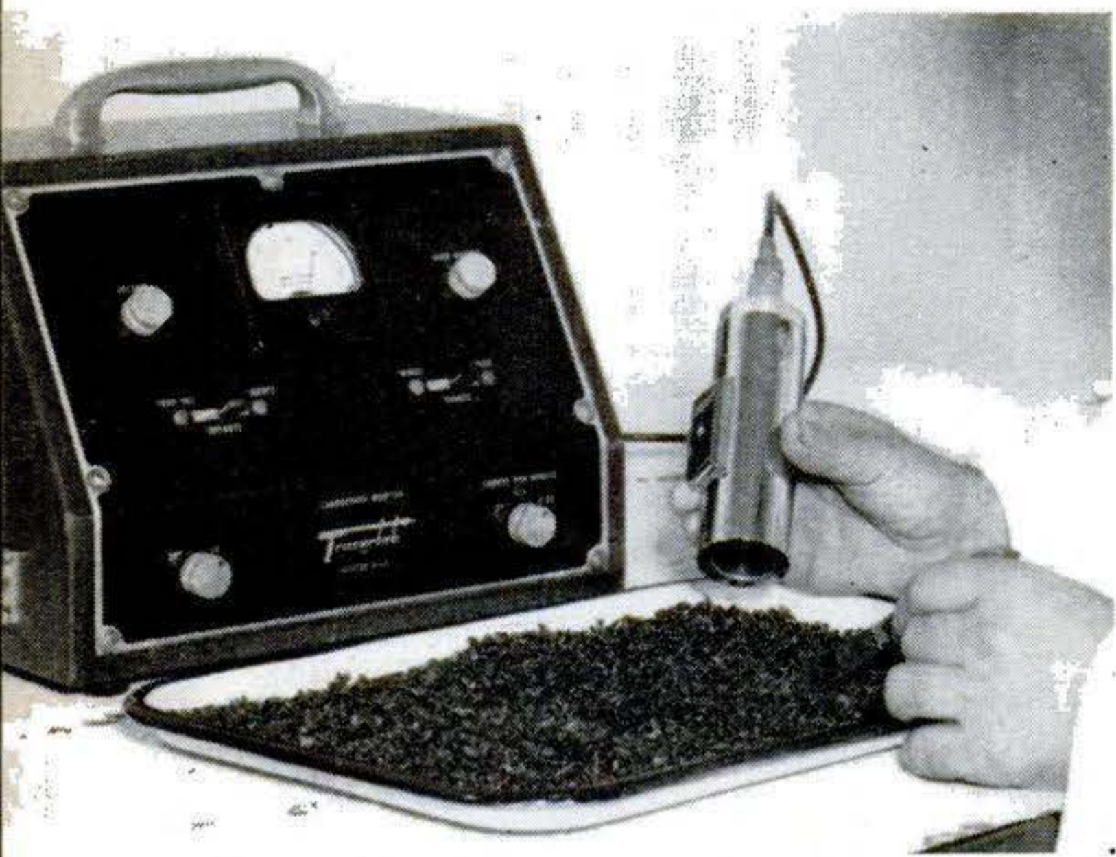
GEIGER COUNTER spots radioactive flies in a trayful caught eight miles from where the feast of "hot" milk was provided. In this manner, researchers follow the flies' wanderings.
